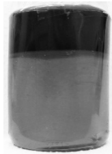
Photograph The top layer was the separated oil and the bottom layer was the glycerol solution appeared in a bottle
