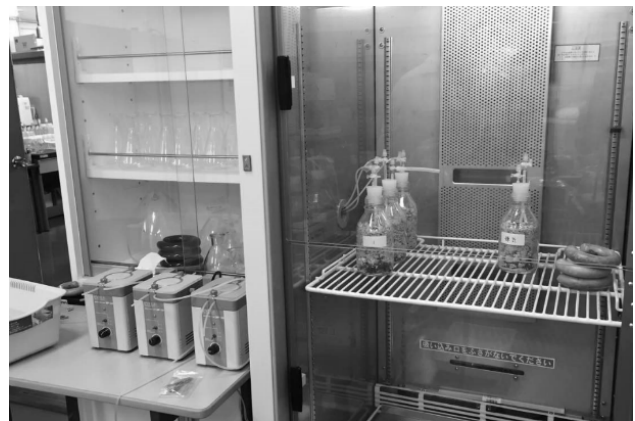
Photo -1 Experimental Status for Hydrogen Sulfide Gas Generation Suppression with Ventilation
